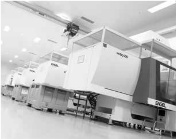
Figure B.5: Cleanroom moulding of fittings and valves.
