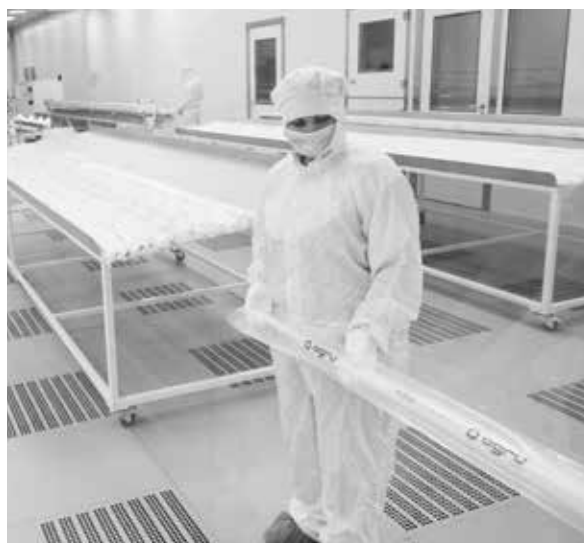
Figure B.8: Triple packaging of PVDF UHP pipes.
