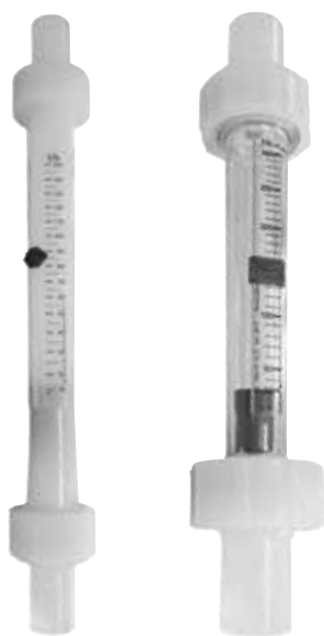
Figure G.94: Flow meter.
